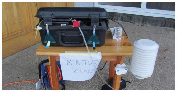
Figure 6: External measuring station
